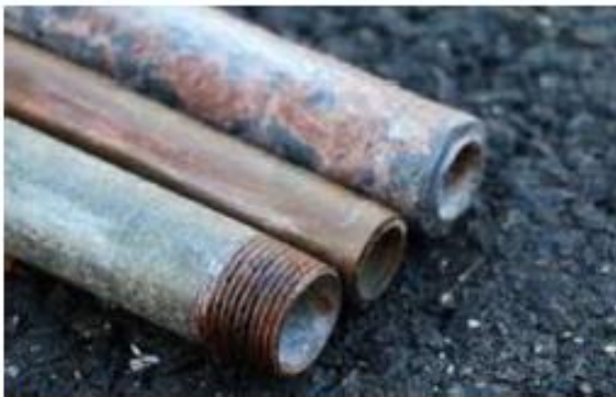
(L-R) Galvanized, Copper, Lead Pipe
